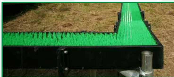
Eel channel pumping station bypass
